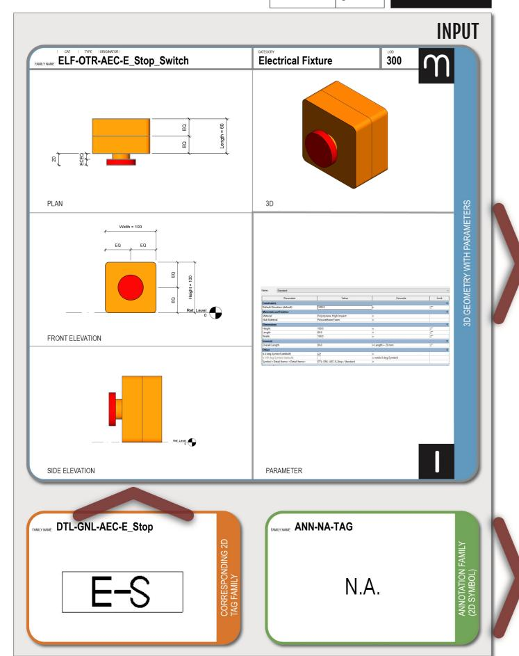
Parameters were setup for size, materials; All parameters are shared parameter; 2-D symbolic lines shown in plans.
