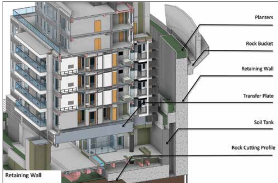
3D Section View of Retaining Wall along Hillside Image courtesy of Sun Hung Kai Properties Limited
