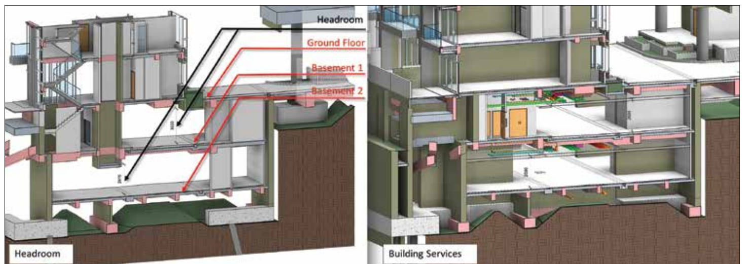
Headroom and Building Services Spaces Coordination and Clash Detection in Model Image courtesy of Sun Hung Kai Properties Limited
