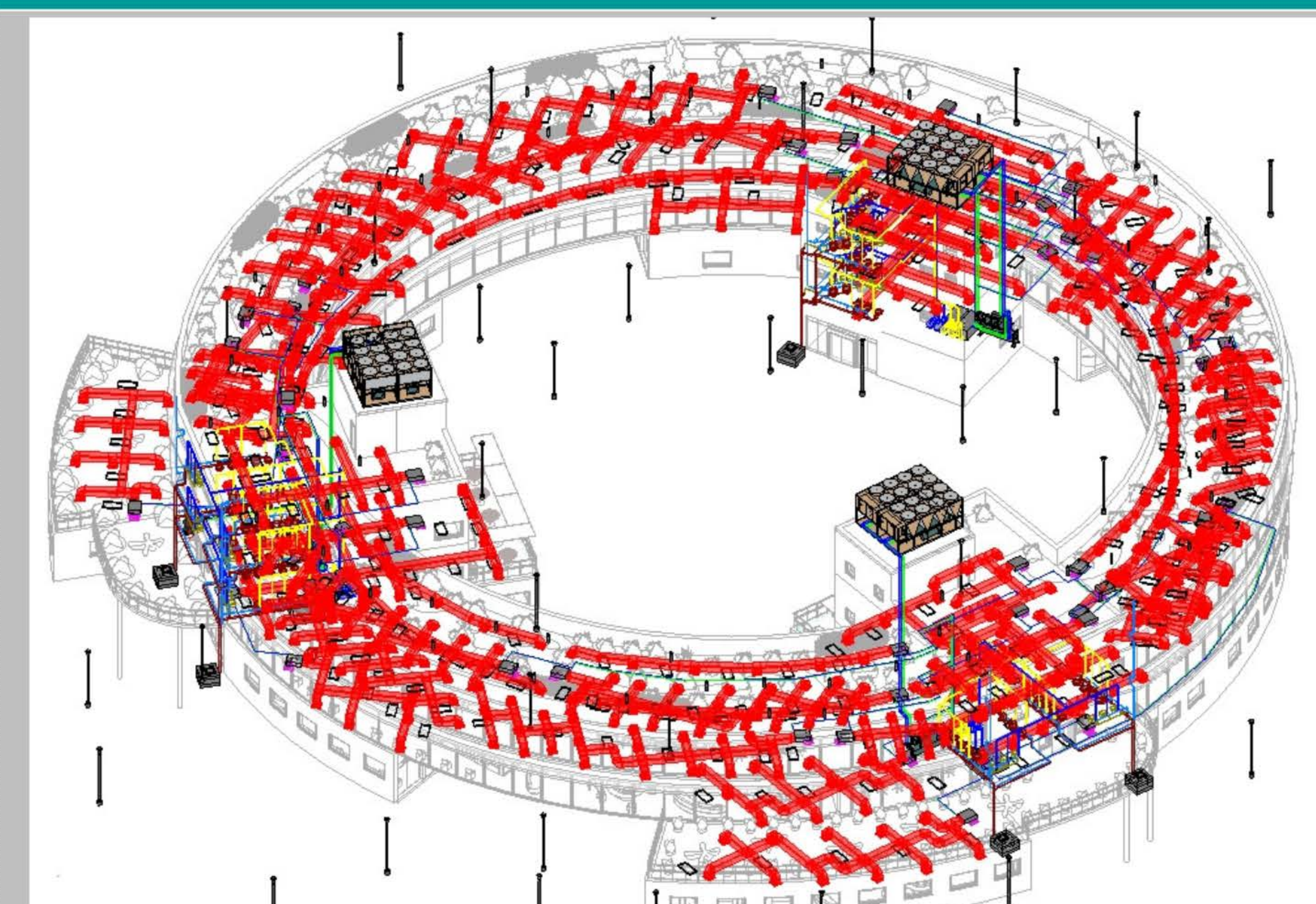
Perspective View: Whole building MEP design of AC system, Drainage system, Plumbing system, Lighting system
